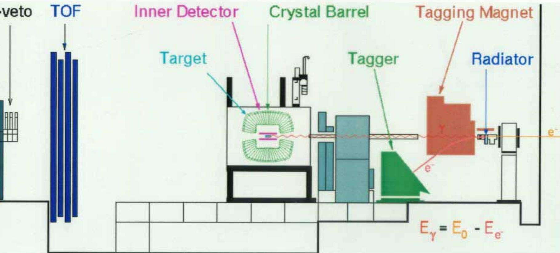
LH<sub>2</sub> target      Crystal Barrel
