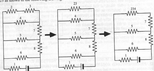
The voltage across resistance 23 and resistor 4 is the same, so these two resistances are in parallel; they can be represented by an equivalent resistance 234. The current through resistance 234 is the same as that through resistor 7, so resistance 234 is in series with resistor 7; they can be represented by an equivalent resistance 2347 as shown in the following figure.
