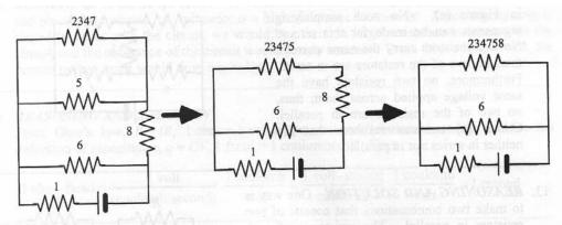
The voltage across 2347 is the same as that across resistor 5; therefore, resistance 2347 is in parallel with resistor 5. They can be represented by an equivalent resistance 23475. Similarly, resistance 23475 is in series with resistor 8, giving an equivalent resistance 234758. Resistance 234758 is in parallel with resistor 6, giving an equivalent resistance 2347586.
