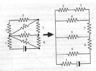
We can see in the redrawn figure that the current through resistors 2 and 3 is the same; therefore, resistors 2 and 3 are in series and can be represented by an equivalent resistance 23 as shown in the following drawing.
